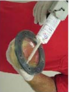
Turn gun down to dispense product. When finished, remove and discard static mixing tube.
